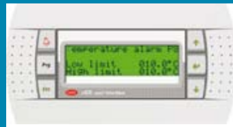
Fig.10 Easy to use microprocessor displays all operating parameters, modes and alarms.
