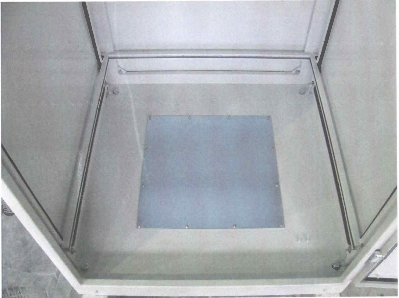
Interior of enclosure after dust test
